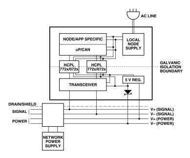
Figure 16. Typical DeviceNet Node.
