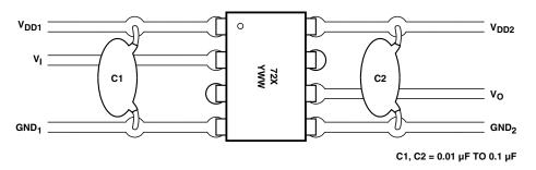
Figure 11. Recommended printed circuit board layout.
