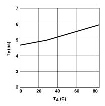
Figure 4. Typical pulse width distortion vs. temperature.
