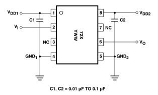
Figure 10. Recommended printed circuit board layout.
