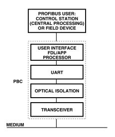
Figure 22. PROFIBUS Controller (PBC).
