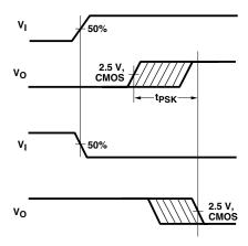
Figure 13. Propagation delay skew waveform.
