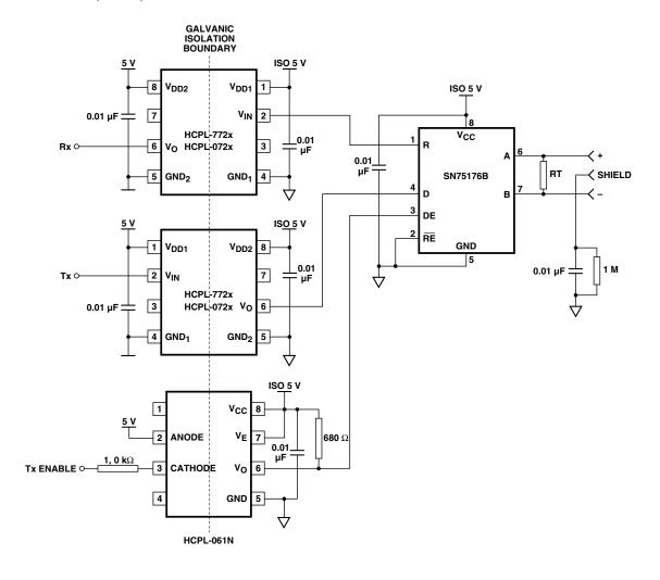
Figure 23. Recommended PROFIBUS application circuit.
