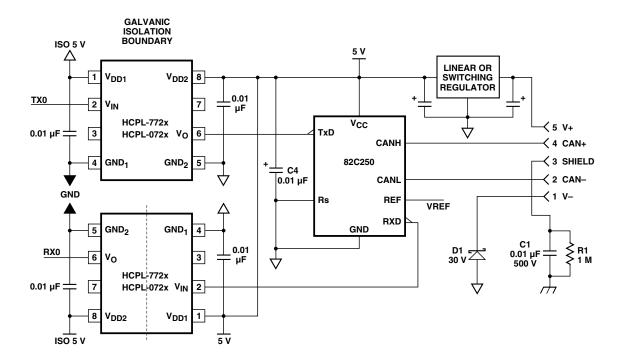
Figure 21. Recommended DeviceNet application circuit.
