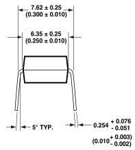
DIMENSIONS IN MILLIMETERS AND (INCHES). \*OPTION 300 AND 500 NOT MARKED.
