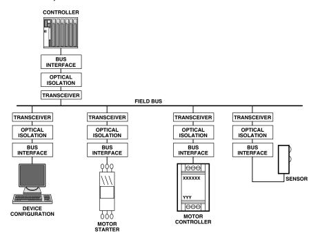
Figure 15. Typical field bus communication physical model.
